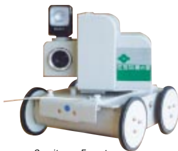
Sumitomo Forestry developed a sub-floor inspection robot to improve maintenance efficiency.
