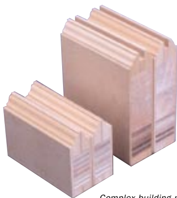
Complex building materials are produced using the MDF and LVL processes of NPIL and KTI, respectively.
