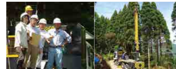
An in-vehicle-type tower yarder in use
