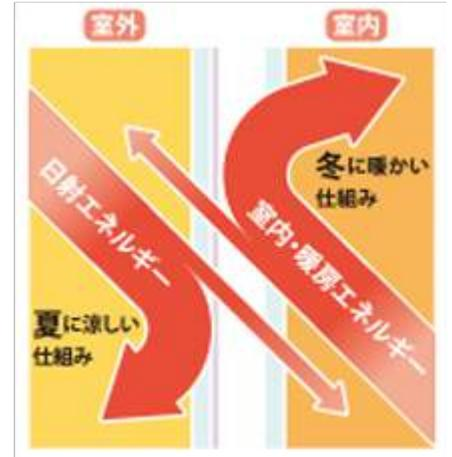
Thermal insulation using low-E glass
