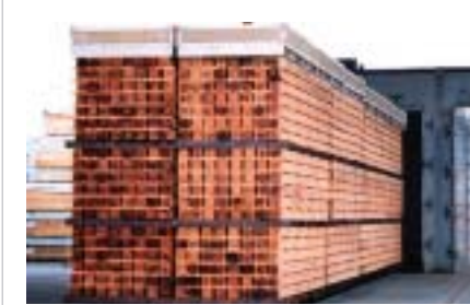
Japanese cedar dried to 15% or less moisture content in the timber drying system
