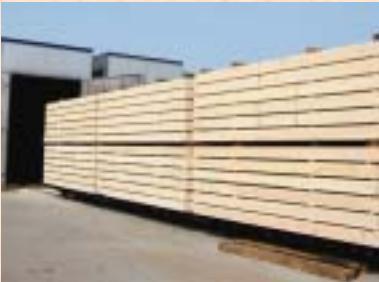
MIZDAS drying system: Whole materials are completely opened to allow exposure to air, and sawn timber is piled up and then put into the dryer.
