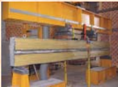
An experiment in concrete foundation reinforcement using band steel and aramid fiber: Aramid fiber is extremely strong and has excellent durability, and is used in cutting-edge fields such as the aerospace industry and aviation.
