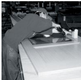
Sumitomo Forestry Crest (Kashima plant) produces interior doors from composite building materials using KTI's planted Falkata wood and MDF made by NPIL.
