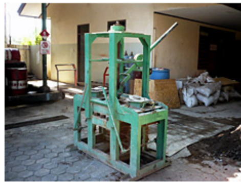
Pressing machines for RPI's roadbed materials
