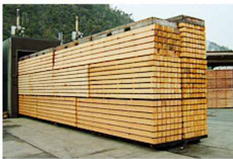
Cypress posts are removed after drying from a kiln equipped with a MIZDAS® system
