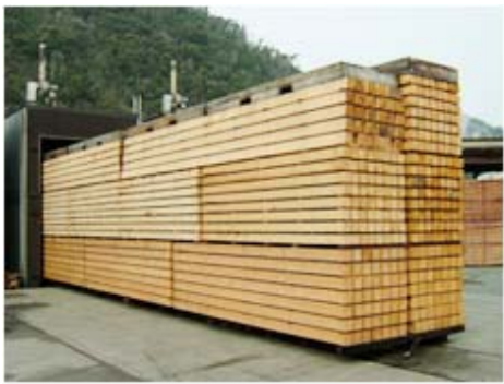
Cypress posts are dried in a kiln equipped with a MIZDAS ® system
