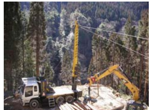
A next-generation tower yarder being used at a Company-owned forest in Kyushu
