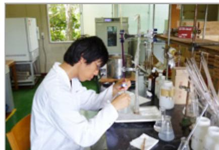
Measuring the COD of effluent
