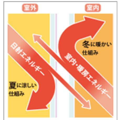
Thermal insulation using low-E glass
