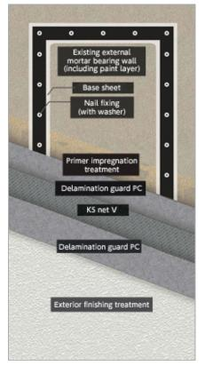
Existing external mortar bearing wall construction method (ReFo.Mo.Wall Construction Method)
