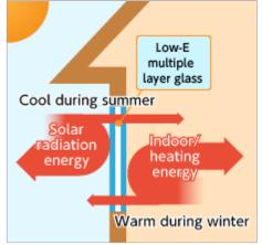
Thermal insulation using low-E glass
