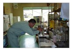
Measuring the COD of effluent
