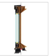
Aluminum and plastic composite frames with high insulation properties
