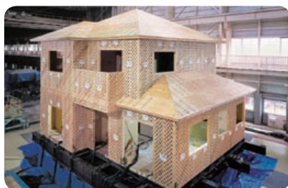
Earthquake resistance testing using actual-size structural models
