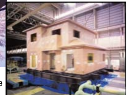
Actual-size vibration testing
