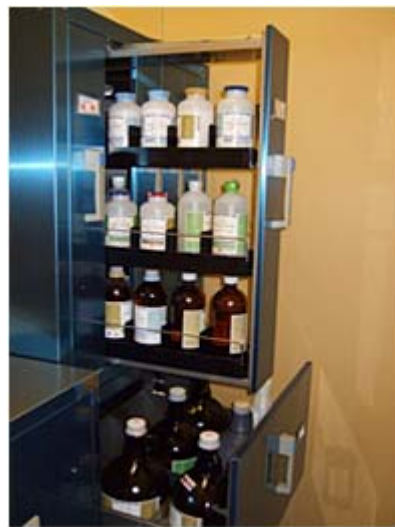
Storage cabinets for poisonous chemicals
