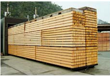
Cypress posts are removed after drying from a kiln equipped with a MIZDAS ® system
