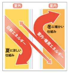
Thermal insulation using low-E glass
