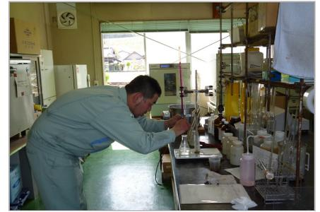
Measuring the COD of effluent
