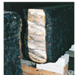
Char layer on the surface of structural material
