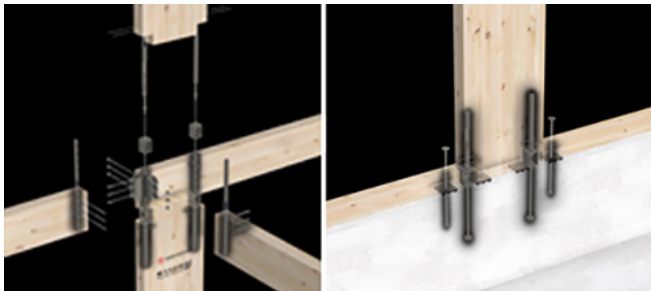
Realizing a Robust Rahmen Structure via Metal-to-Metal Joints
