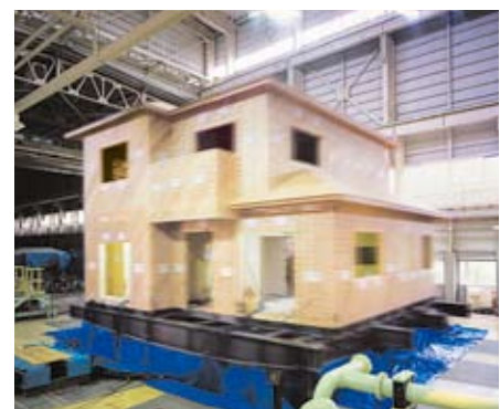
Testing product strength by applying pressure on a full-scale model
