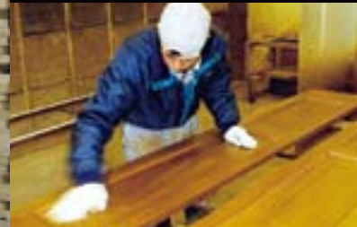
Door coatings are painstakingly checked (Sumitomo Forestry Crest)
