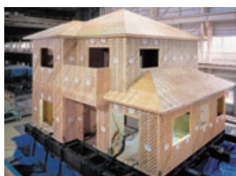
3D vibration test at Tsukuba Research Institute
