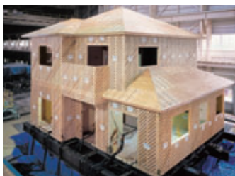
3D vibration test at Tsukuba Research Institute
